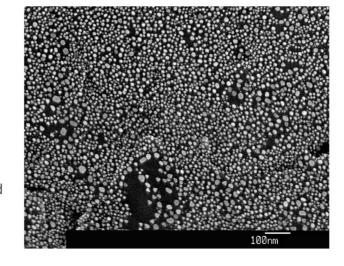
the 'standard' Agar gold on carbon specimen, AGS168. Many of the instructions given on the AGS168 technical leaflet apply also to these ultra-high resolution test specimens, but it should be noted that the instrumental magnification required to resolve the smaller particles, will be higher.
